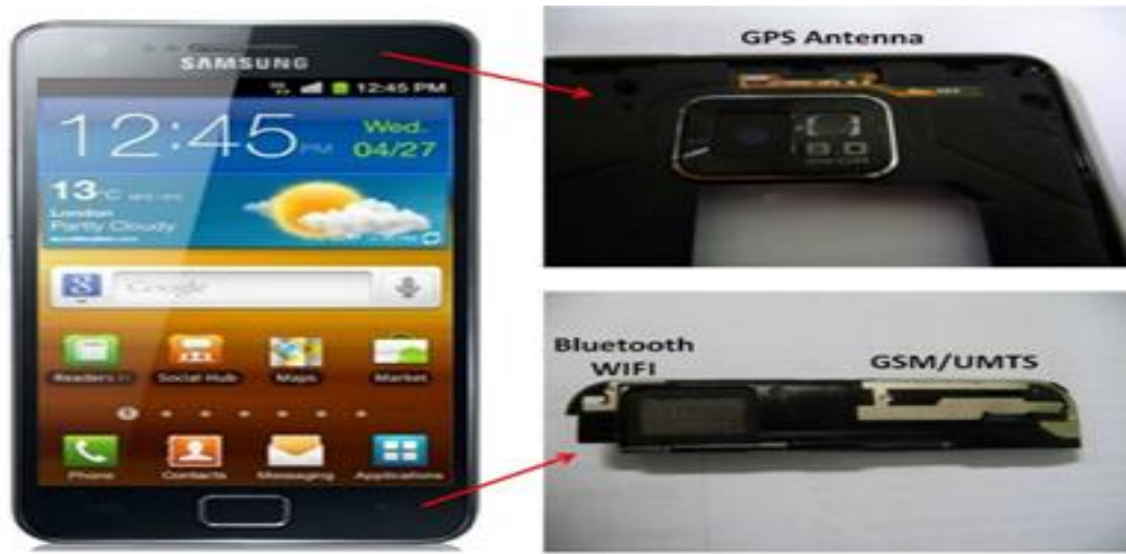
Antenna Placement of Samsung Galaxy SII
